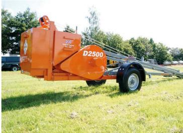
Dando 2000, 2500 and 3000 cable percussive drilling rigs are frequently used to construct boreholes for both geotechnical and environmental investigation. The system of drilling can produce boreholes between 150 and 450mm in diameter, to depths of up to 50m, depending on the underlying geology.
