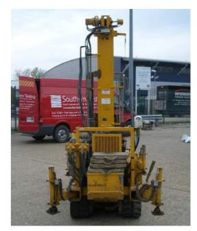
We operate a tracked, self-propelled Sedi Drill 90 rotary investigation rig, which incorporates a Lutz-Data-Logger in order to record the rate of drilling and thrust and torque pressures. .
