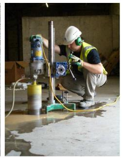
We operate a range of rigs to provide core samples from various concrete surfaces or structures so that investigation, laboratory testing or analysis can take place.
