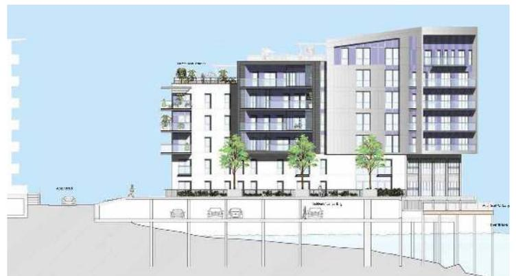
The British Geological Survey map for the area indicated the underlying soils to comprise Alluvium over Gravel over Chalk, which, due to its soft and variable nature, could give rise to many construction problems. The investigation revealed a significant thickness of the Alluvial Deposits (soft clay and peat) to depths of up to 8m over 2-3m of gravel with chalk at depth.
