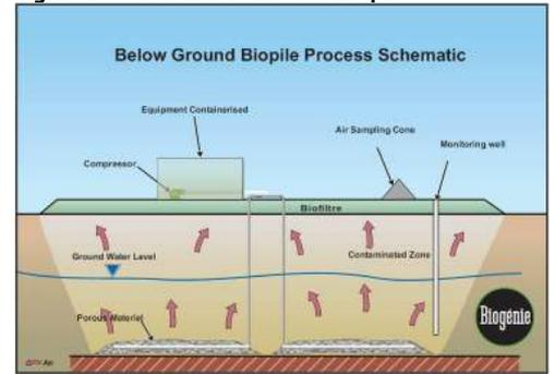
Figure 8 – In Situ Biopile Collector Pipework
